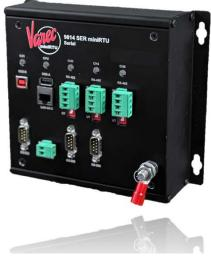
The standard, built-in OPC UA server communicates natively over standard internet protocols. This allows human-machine interface (HMI) applications to read data from the 9810 miniRTU. The 9810 miniRTU is also compatible with a wide range of systems, including legacy Varec systems, using RS-232 and RS-485 standards.
