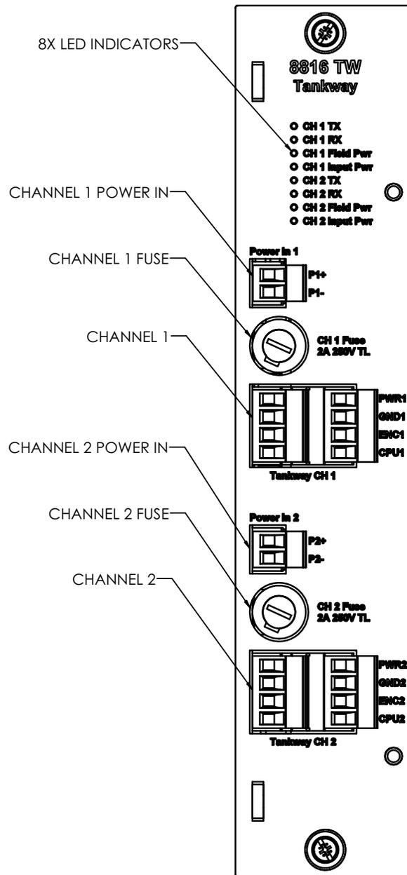
Figure 9-1: 8816 TW Tankway Module Face Plate
