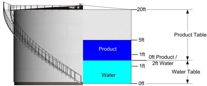
This example shows how the product and water volumes are calculated when the water level is equal to the top point in the water table.
