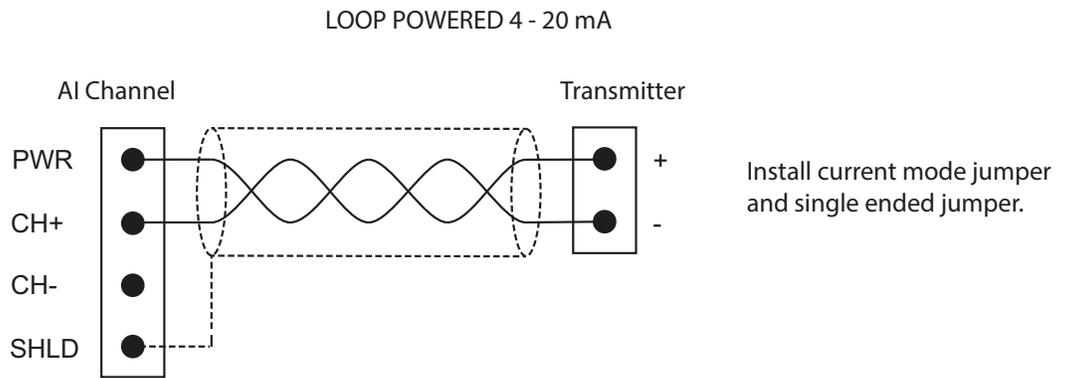
Figure 11-5: 8818 Analog Loop Powered 4-20 mA Wiring
