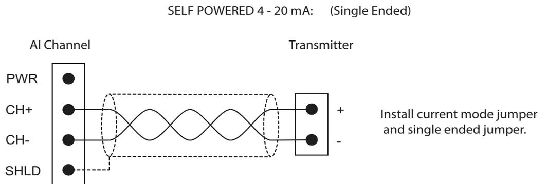
Figure 11-6: 8818 Analog Self-Powered 4-20 mA (Single Ended) Wiring
