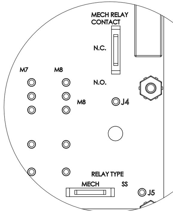
Figure 6-10: 8813 Digital Input/Output Module Watchdog Switch Details
