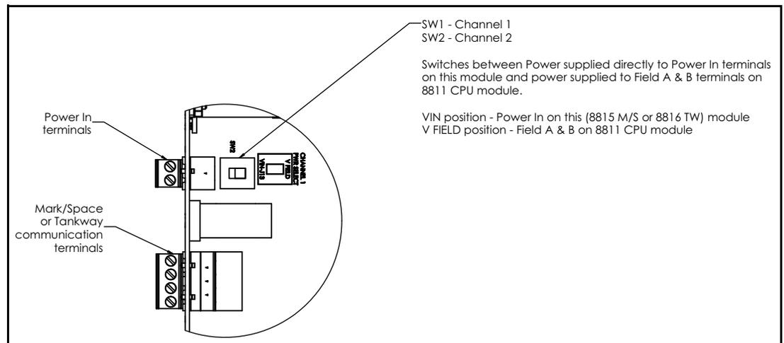
Figure 9-4: 8816 Tankway Module Terminals and Switches Closeup
