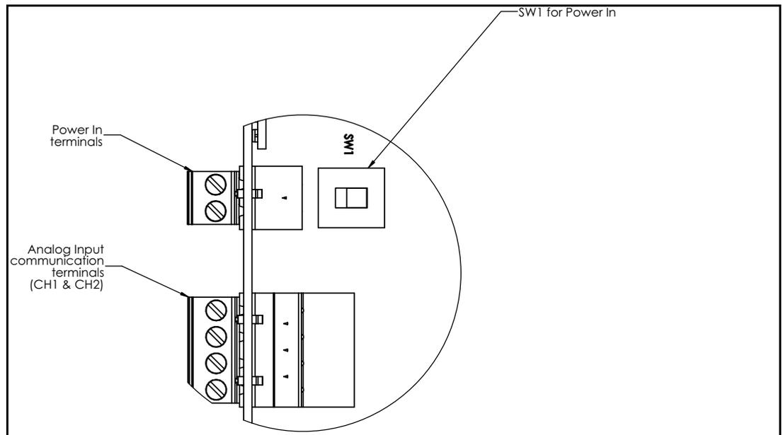
Figure 11-4: 8818 Analog Input Module Terminals and Switch Closeup
