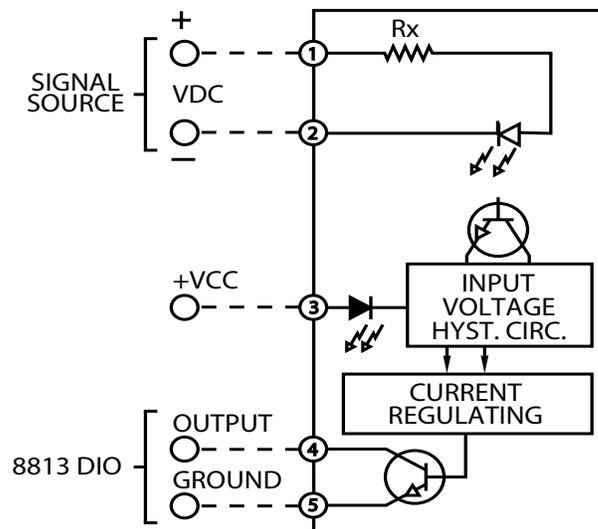
Figure 6-3: 8813 Digital DC Input Solid-state Relay
