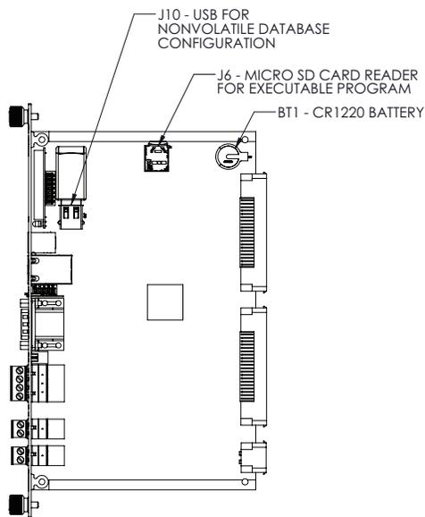
Figure 4-2: 8811 CPU Module Side View
