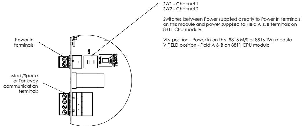
Figure 8-3: 8815 Mark/Space Module Terminals and Switches Closeup
