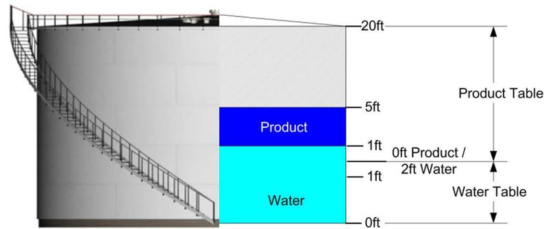
Example 2 shows how the product and water volumes are calculated when the water level is higher than the top point in the water table
