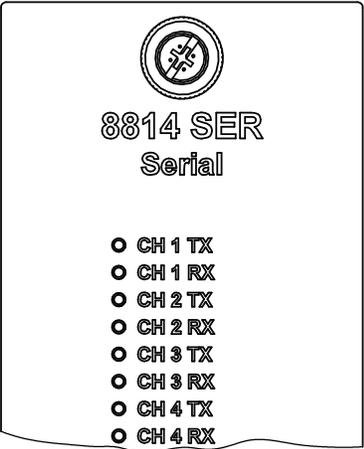
Figure 7-3: 8814 Serial Module LED Indicators
