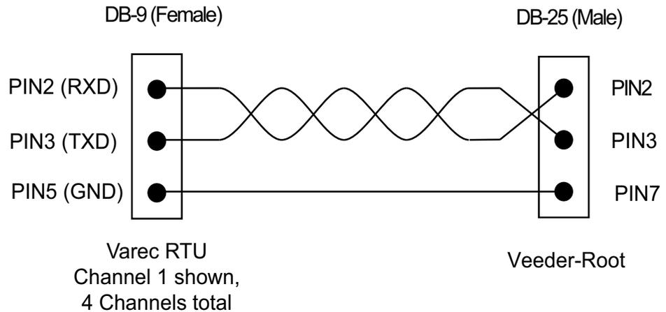
Figure 7-6: 8814 Serial Module Veeder-Root Field Wiring
