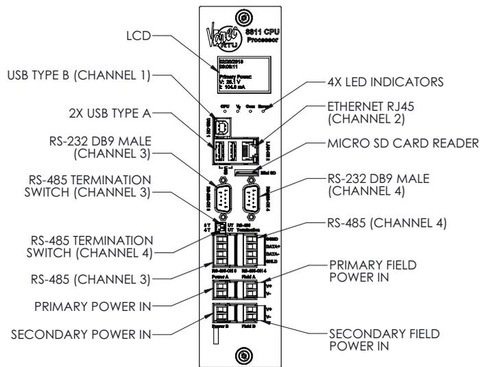
Figure 4-1: 8811 CPU Module Face Plate
