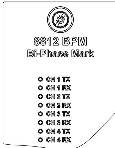
Figure 5-3: 8812 Bi-Phase Mark Module LED Indicators
