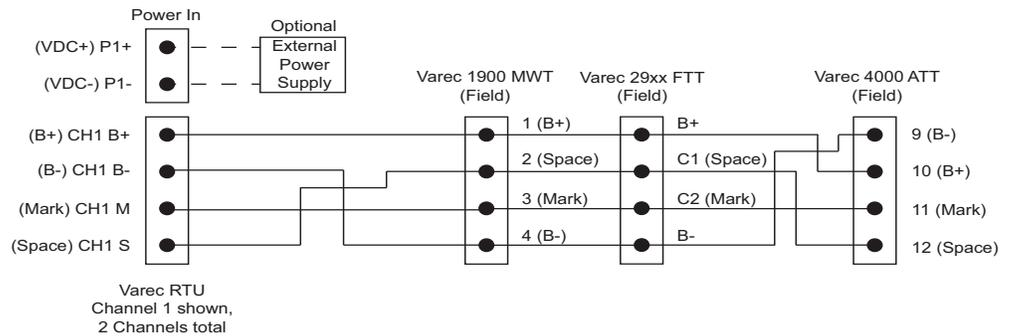
Figure 8-6: 8815 Mark/Space Module Field Wiring
