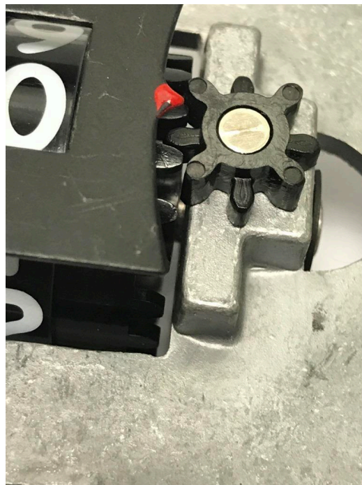
Figure 3-20: Pinion counter wheel alignment on whole numbers
