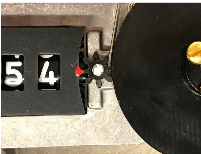
Figure 33: Measure counter spacing with feeler gauge at pinion
