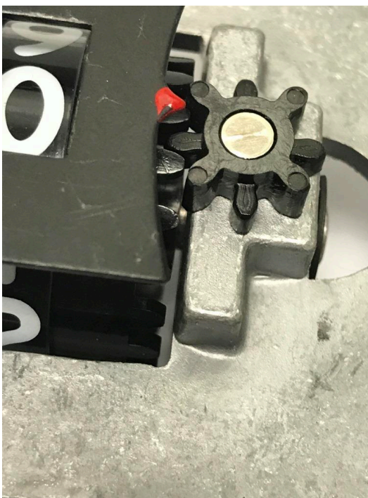
Figure 34: Pinion counter wheel alignment on whole numbers
