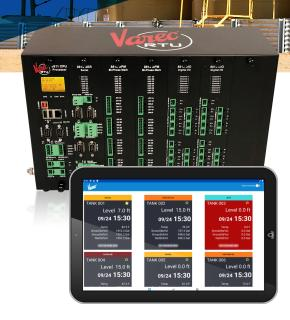
The Android Display is an application specifically designed to provide local visualization of process data from an 8810 remote terminal unit (RTU). This data is rendered on a portable tablet or mounted panel display running the Android operating system.
