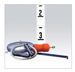
The 6600 Liquid Level Indicator (LLI) is a tank side device. A float inside the tank is connected to an indicator in a clear tube mounted outside of the tank. The indicator moves up and down based on the level of product in the tank.
