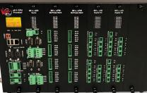
With the CPU module serving as the base functionality for the 8810 RTU, all logic and protocols are handled seamlessly, meaning there is only one firmware application for the entire unit.
