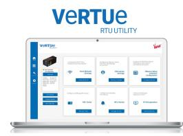
Vertue is optimized for bulk liquid applications and has efficiency tools built in for common actions to streamline the configuration process. Vertue can be configured using any workstation on the network and supports offline configuration.
