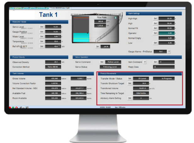
Movement data is also available for each tank on the tank detail screen.
