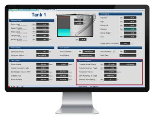
Movement data is also available for each tank on the tank detail screen.
