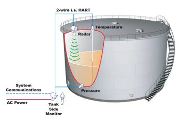
Example tank gauging system using the 4590 Tank Side Monitor and 4532/4539 Average Temperature Converter
