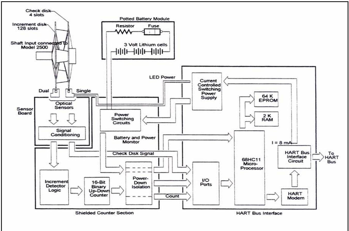
Figure 6-1: 4110 HLE Block Diagram
