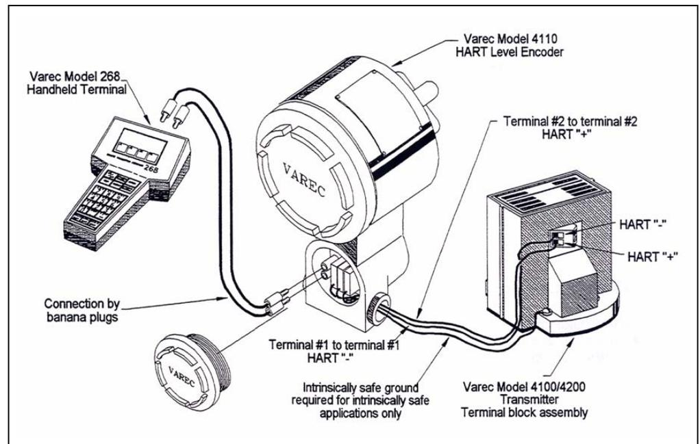
Figure 2-4: 4110 HLE Wiring Connections
