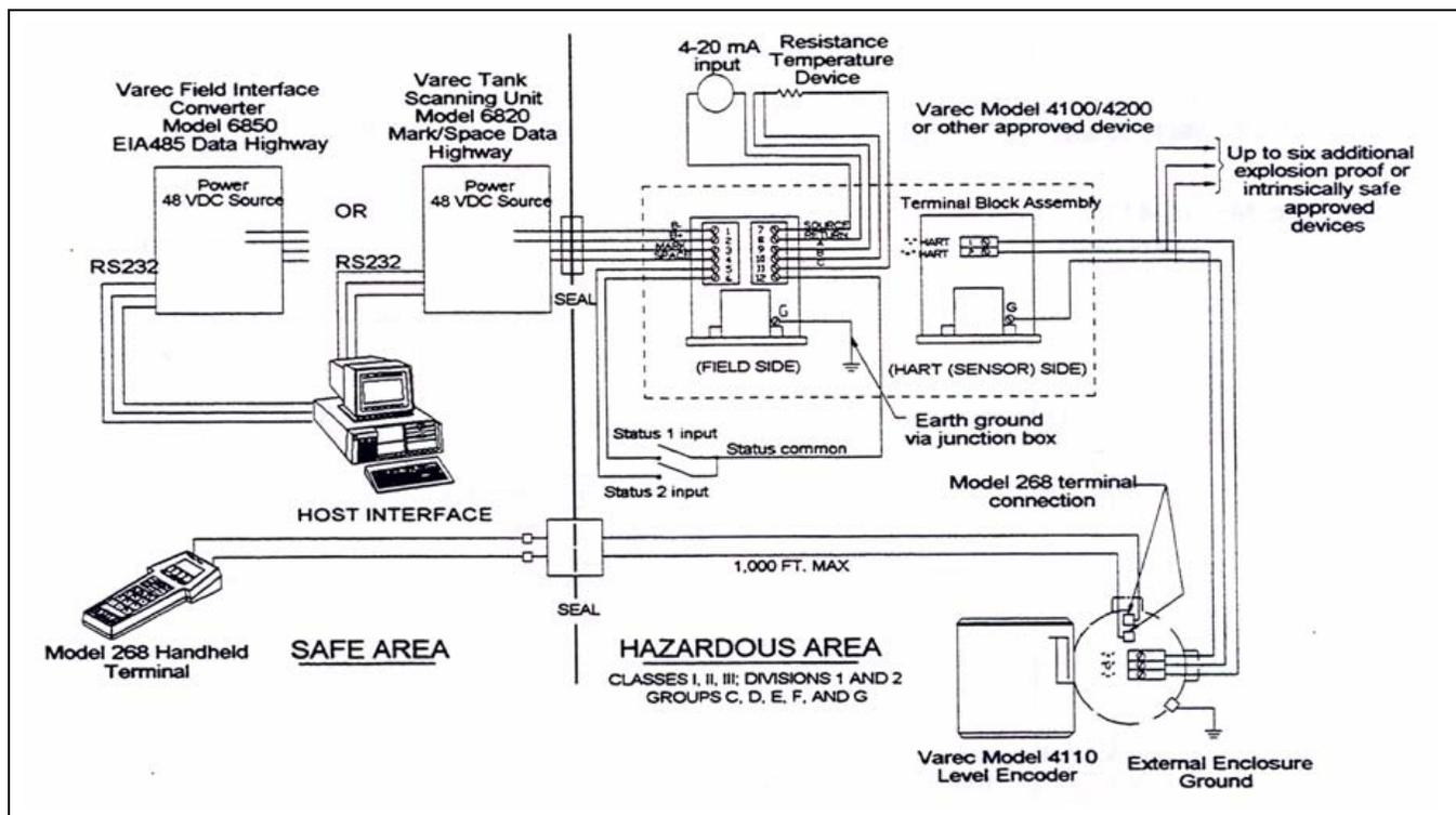
Figure 2-2: Typical System Installation
