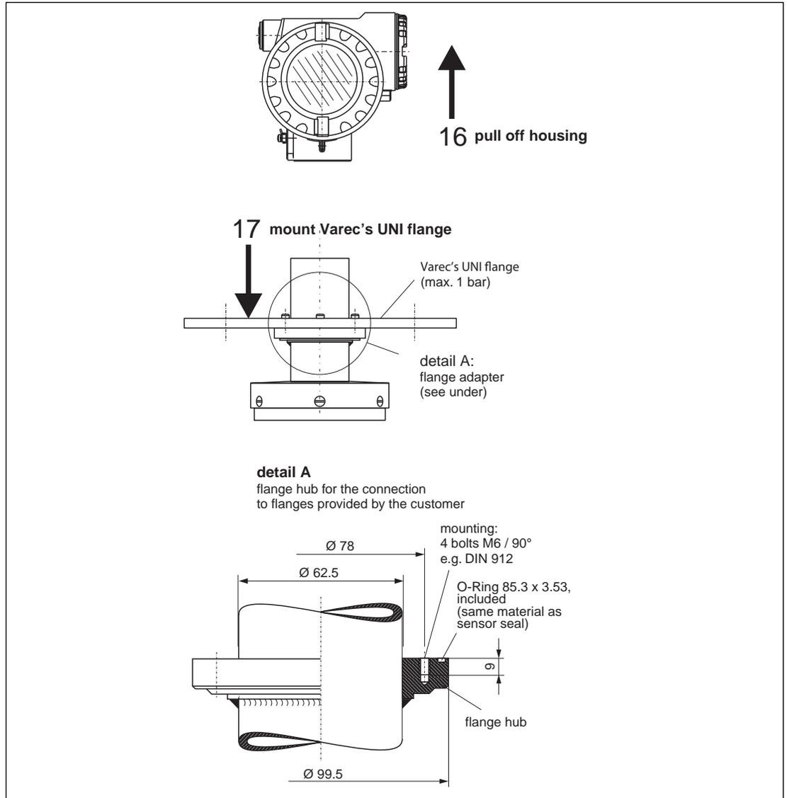
Figure 4-14: Preparation for the Installation of the Varec UNI Flange, cont'd
