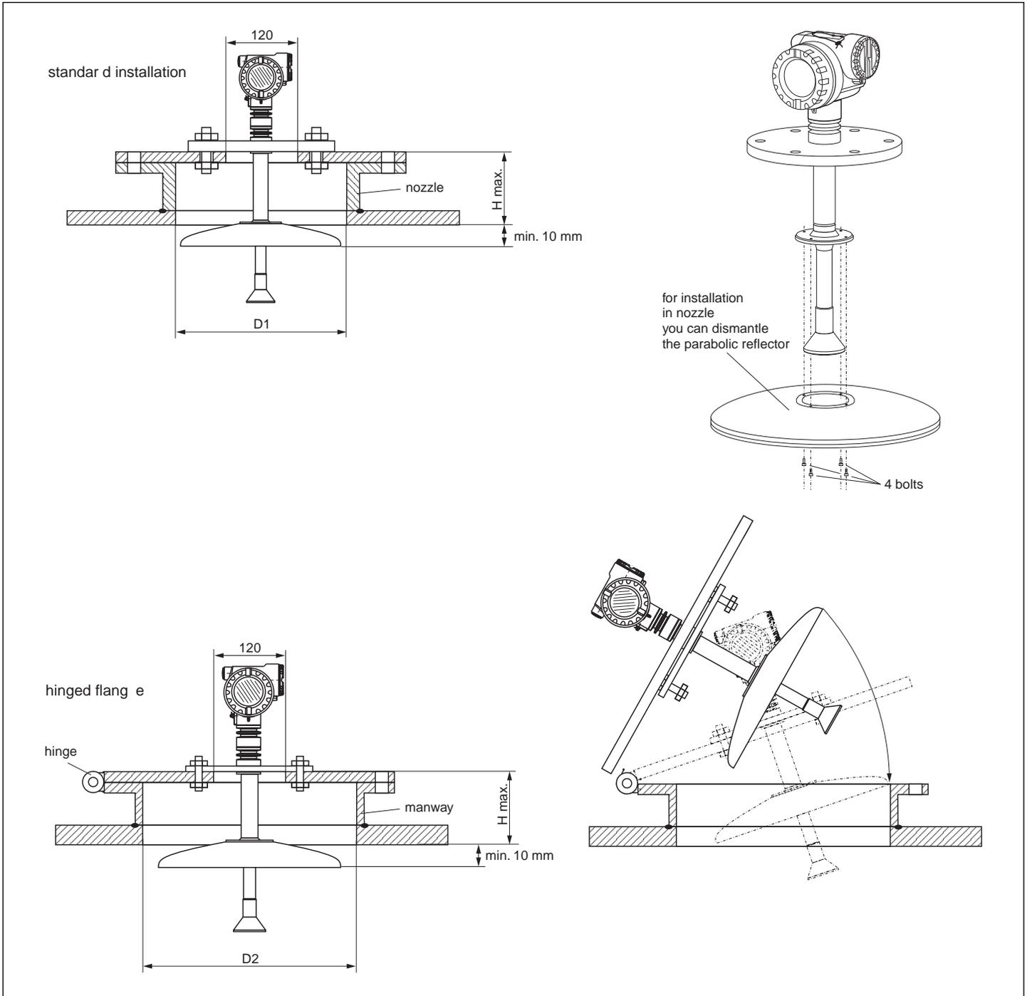
Figure 4-10: Examples for Installation in a Manway
