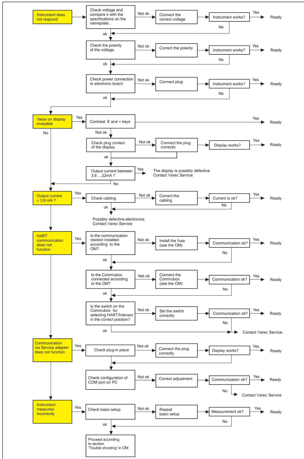
Figure 10-1: Troubleshooting the 7500 Series Radar Tank Gauges
