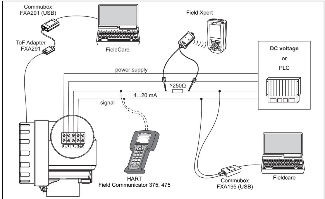
Figure 5-4: HART Connection with Other Supplies
