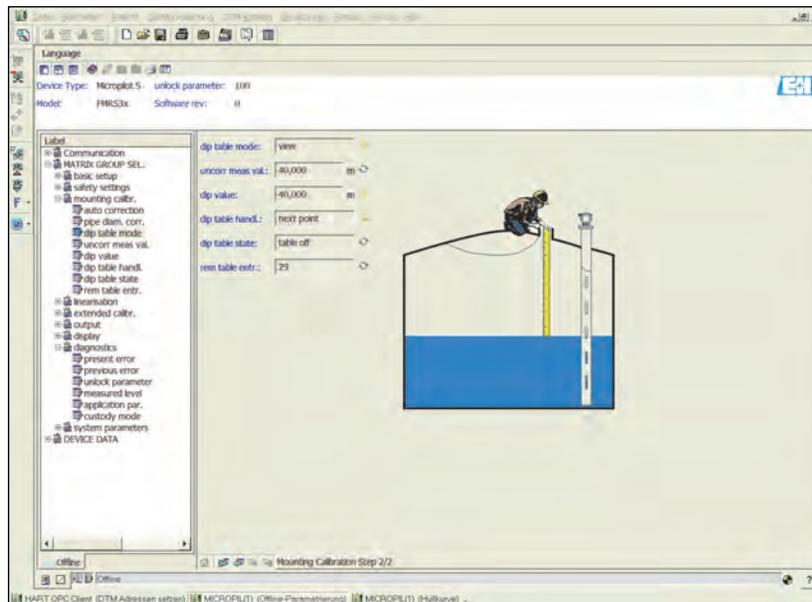
Figure 7-19: 7500 Series Radar Tank Gauges – Mounting Calibration (Step 2/2)
