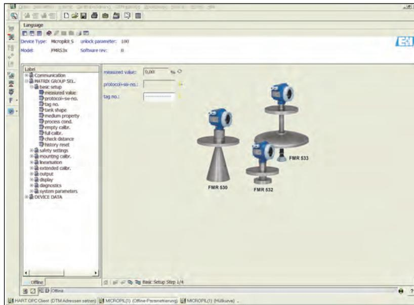
Figure 7–10: 7500 Series Radar Tank Gauges – Basic Setup (Step 1 /5)
