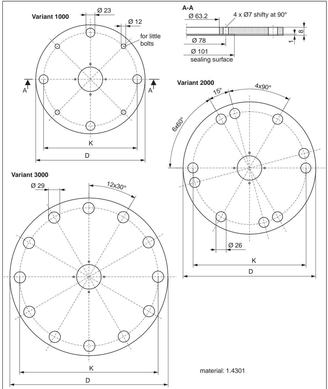
Figure 4-12: Installation with Varec's UNI Flange
