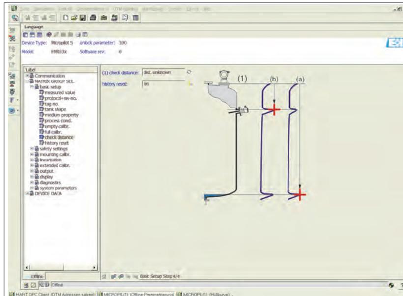
Figure 7-16: 7500 Series Radar Tank Gauges– Basic Setup (Step 7)
