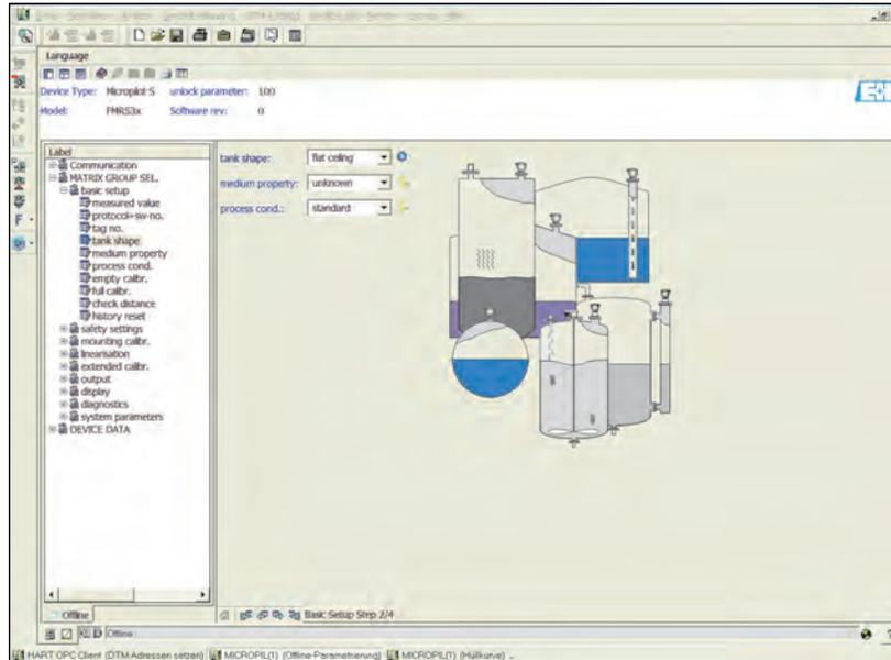
Figure 7-11: 7500 Series Radar Tank Gauges – Basic Setup (Step 2/5)
