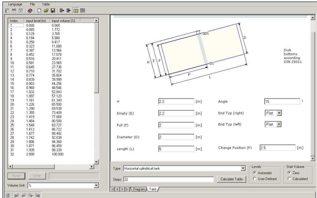
Figure 6-7: 7500 Series Radar Tank Gauges Tank Linearization
