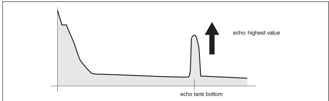
Figure 10-4: Vessel empty, no interference echo
