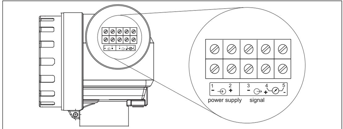
Figure 5-3: Housing with a Separate Terminal Compartment
