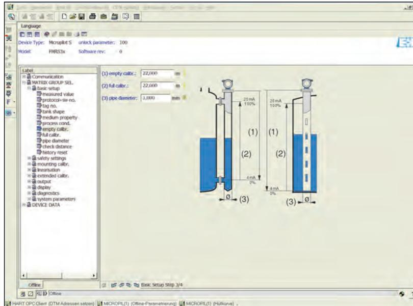
Figure 7-14: 7500 Series Radar Tank Gauges – Basic Setup (Step 5/5)
