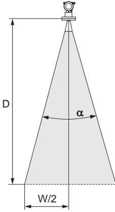
The diagram shows a radar antenna at the top, emitting a conical beam. The vertical distance from the antenna to the tank bottom is labeled  $D$ . The beam angle is labeled  $\alpha$ . The horizontal distance from the centerline to the edge of the beam at the tank bottom is labeled  $W/2$ .
