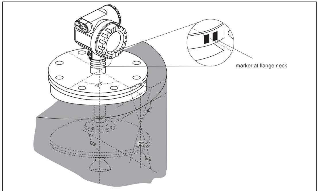
Figure 4-9: Optimum Mounting Position
