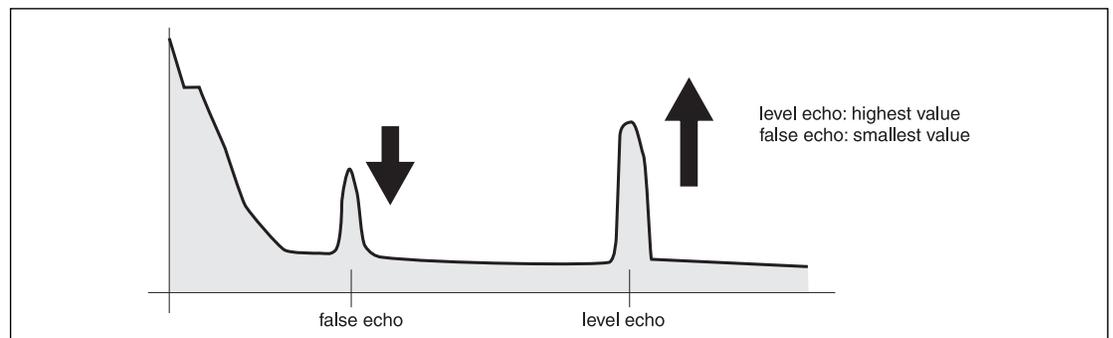
Figure 10-3: Vessel Partly Full, Interference Echo Obtained
