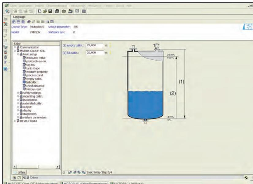
Figure 7-15: 7500 Series Radar Tank Gauges – Basic Setup (Step 6)
