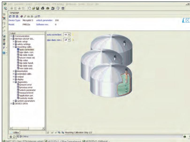
Figure 7-18: 7500 Series Radar Tank Gauges – Mounting Calibration (Step 1 /2)
