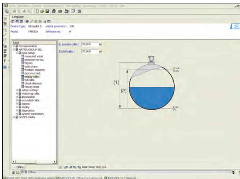
Figure 7-13: 7500 Series Radar Tank Gauges – Basic Setup (Step 4/5)
