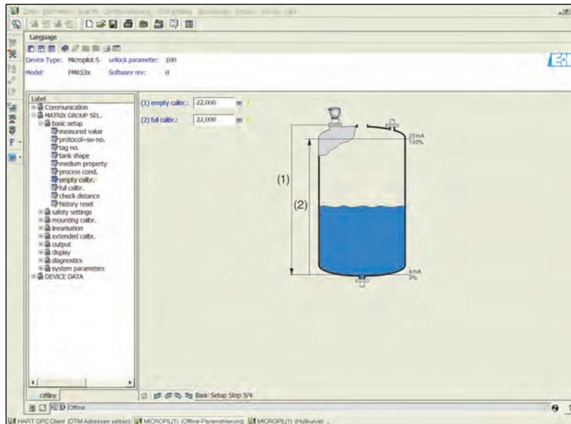
Figure 7-12: 7500 Series Radar Tank Gauges – Basic Setup (Step 3/5)
