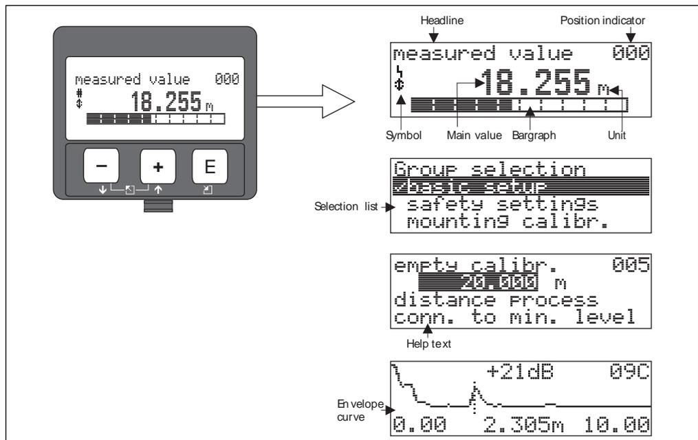
Figure 6-4: Liquid Crystal Display (LCD)
