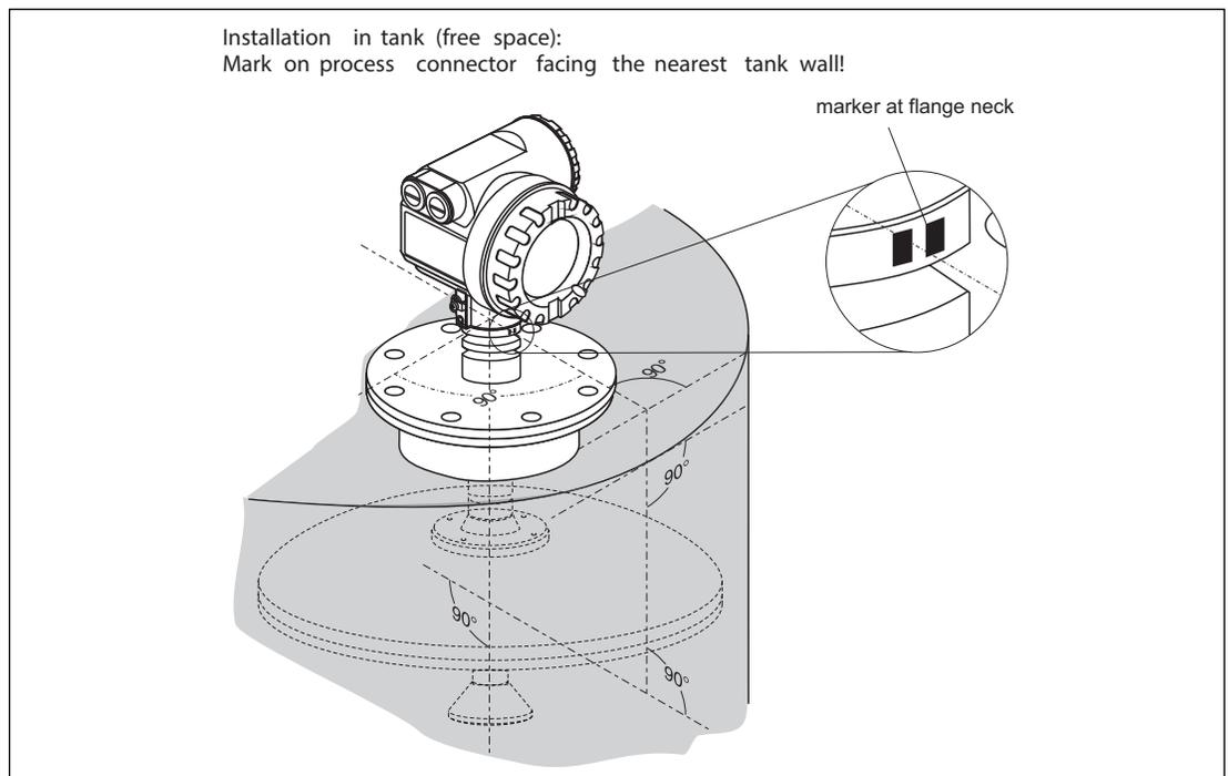
Figure 4-1: Installation Orientation
