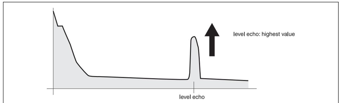
Figure 10-2: Vessel Partly Full, No Interference Echo Obtained
