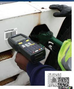
The system identifies the individual GSE by scanning any type of barcode on the equipment. When the system is commissioned, you decide which type of barcode will be used. This can be a new barcode label placed on the equipment, or an existing barcode already located on the equipment.
