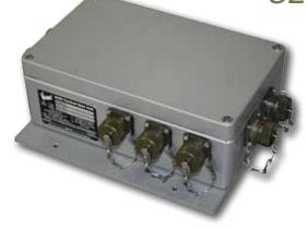
The 8240 Tactical Data Unit (TDU) collects pressure, temperature and flow measurements from connected field devices, such as the Varec 7660 Tactical Fuel Gauge (TFG) or a Tactical Flow Meter (TFM). It calculates observed fuel volumes and performs the collapsible tank mapping process. All data is transferred to the TacFuels® Tactical Mobile Computer for inventory management and accounting.
