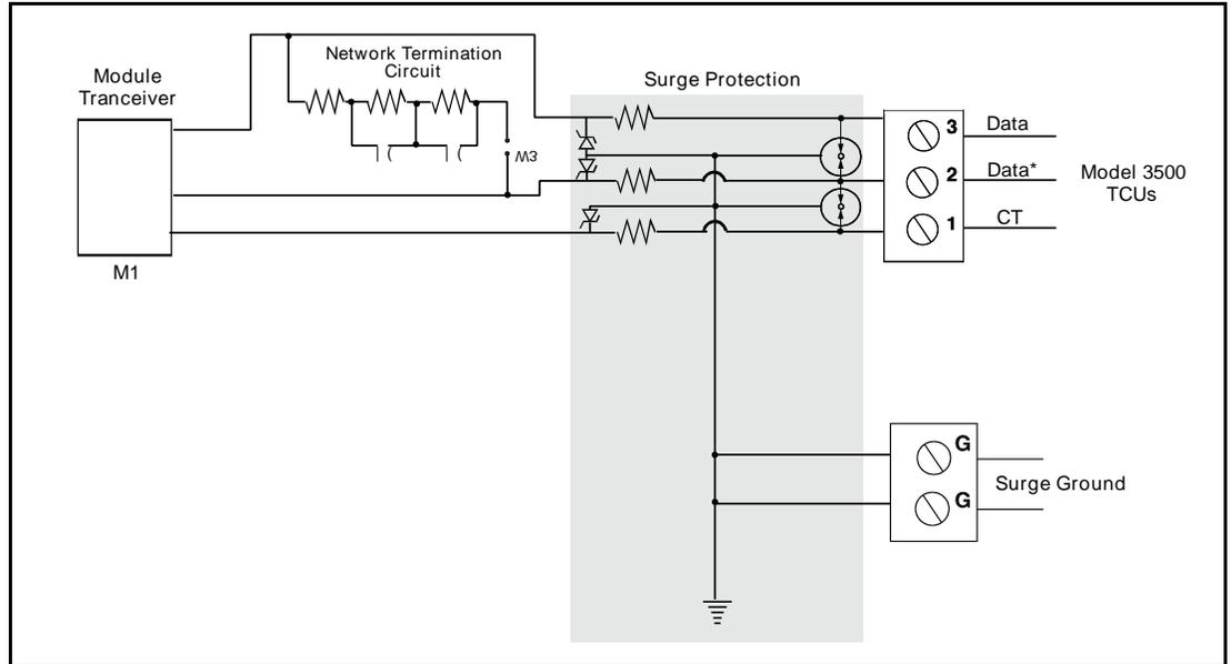
Figure 3-3: Input Circuit
