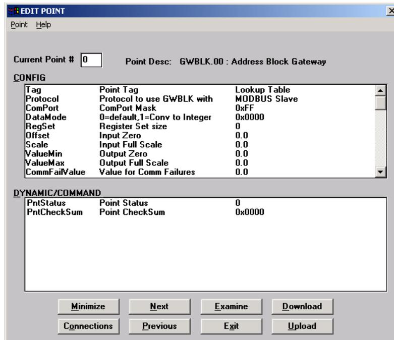
Figure 4-2: Adding a GWBLK point in View RTU
