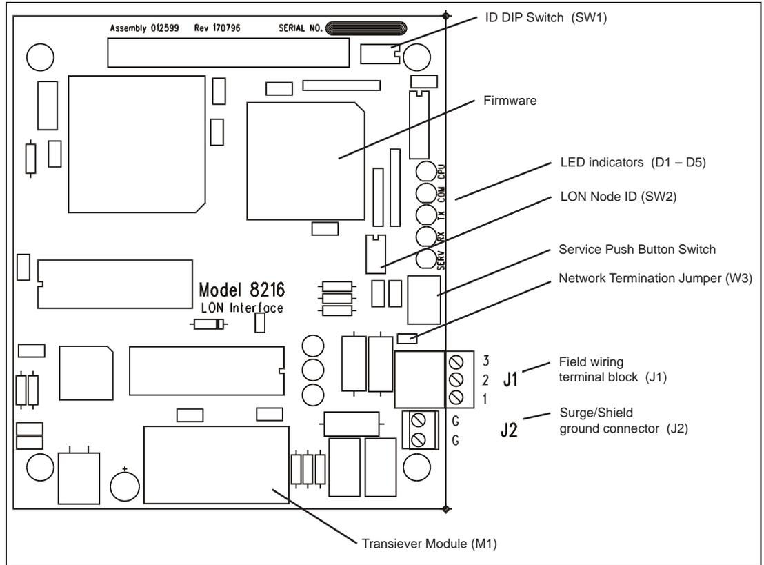
Figure 3-1: Echelon LON Tank Gate Interface Module
