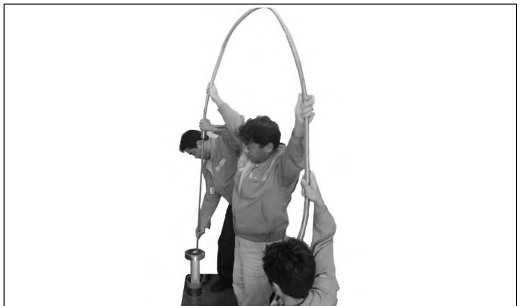
Figure 4-7: Flexible tube / WB probe installation
