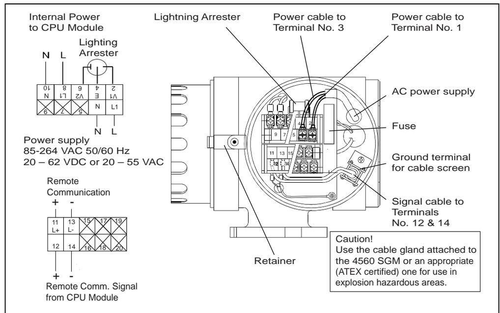
Figure 4-1: Electrical connection of the 4560 SGM
