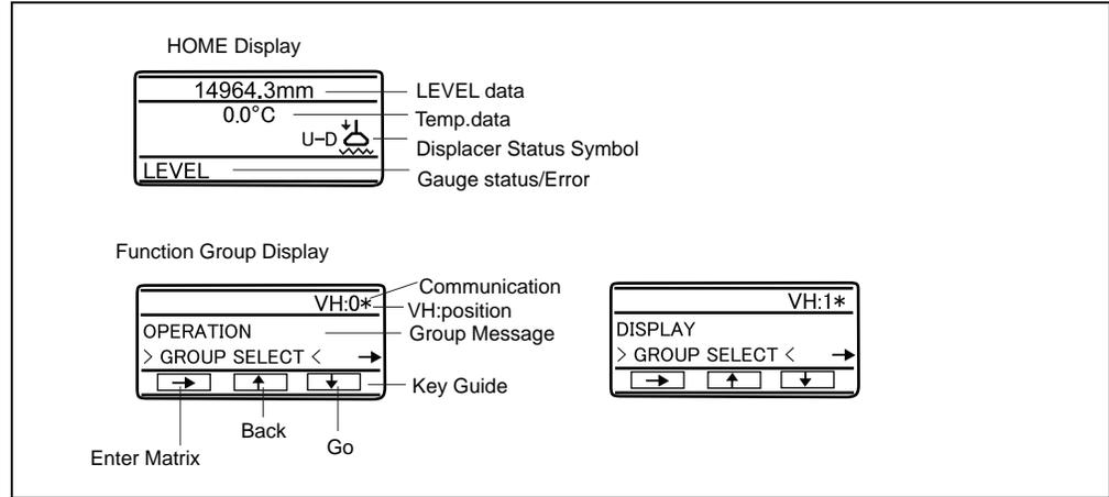
Figure 5-2: LCD display functions
