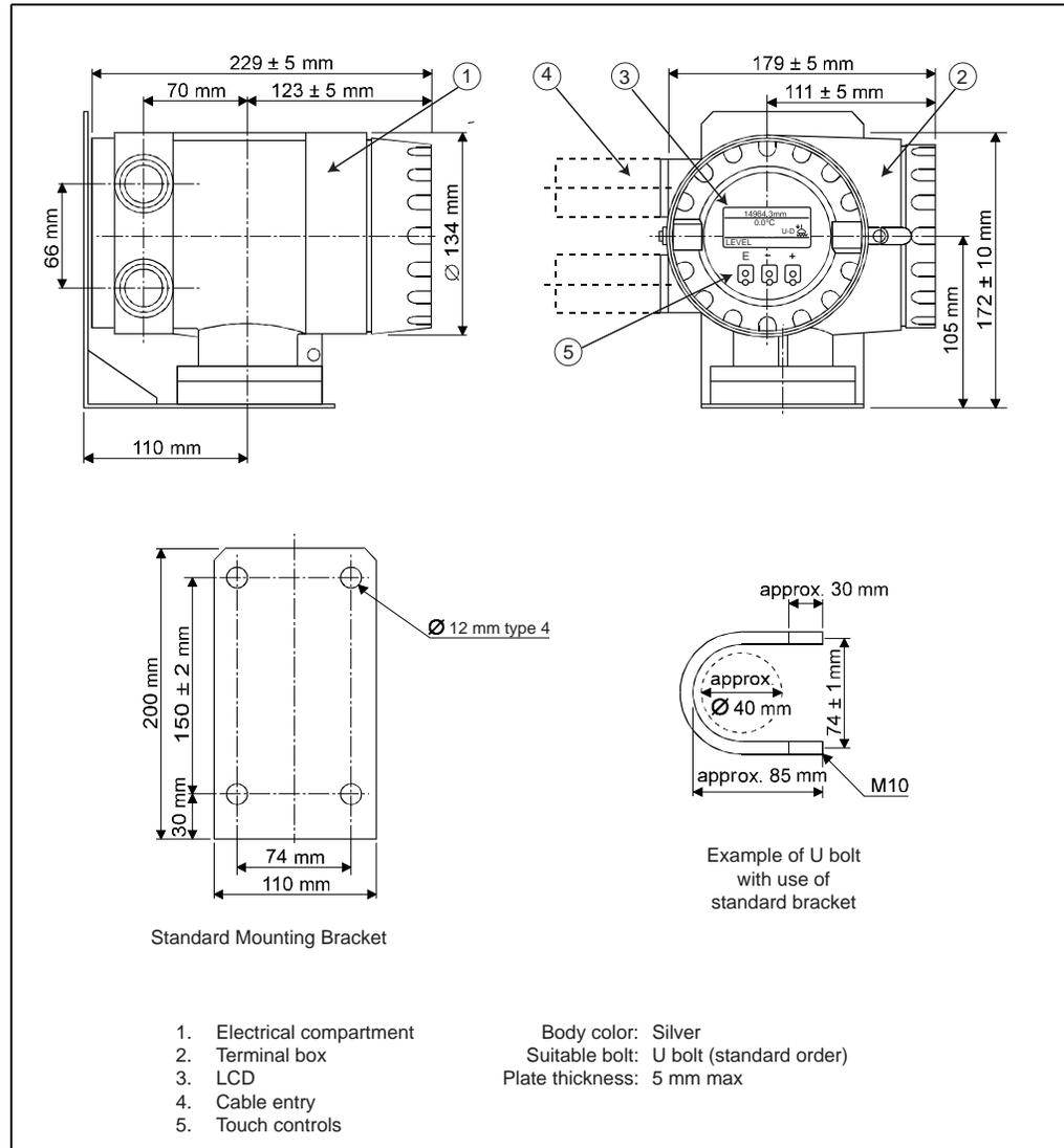
Figure 2-1: Dimensions of the 4560 SGM
