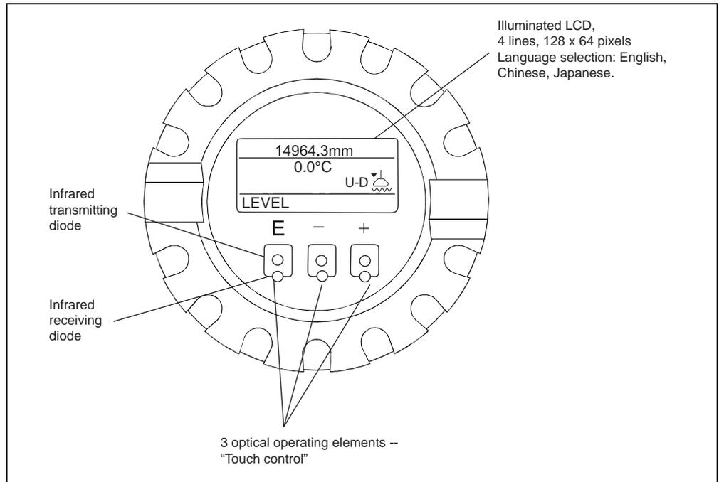
Figure 5-1: Display and operating elements
