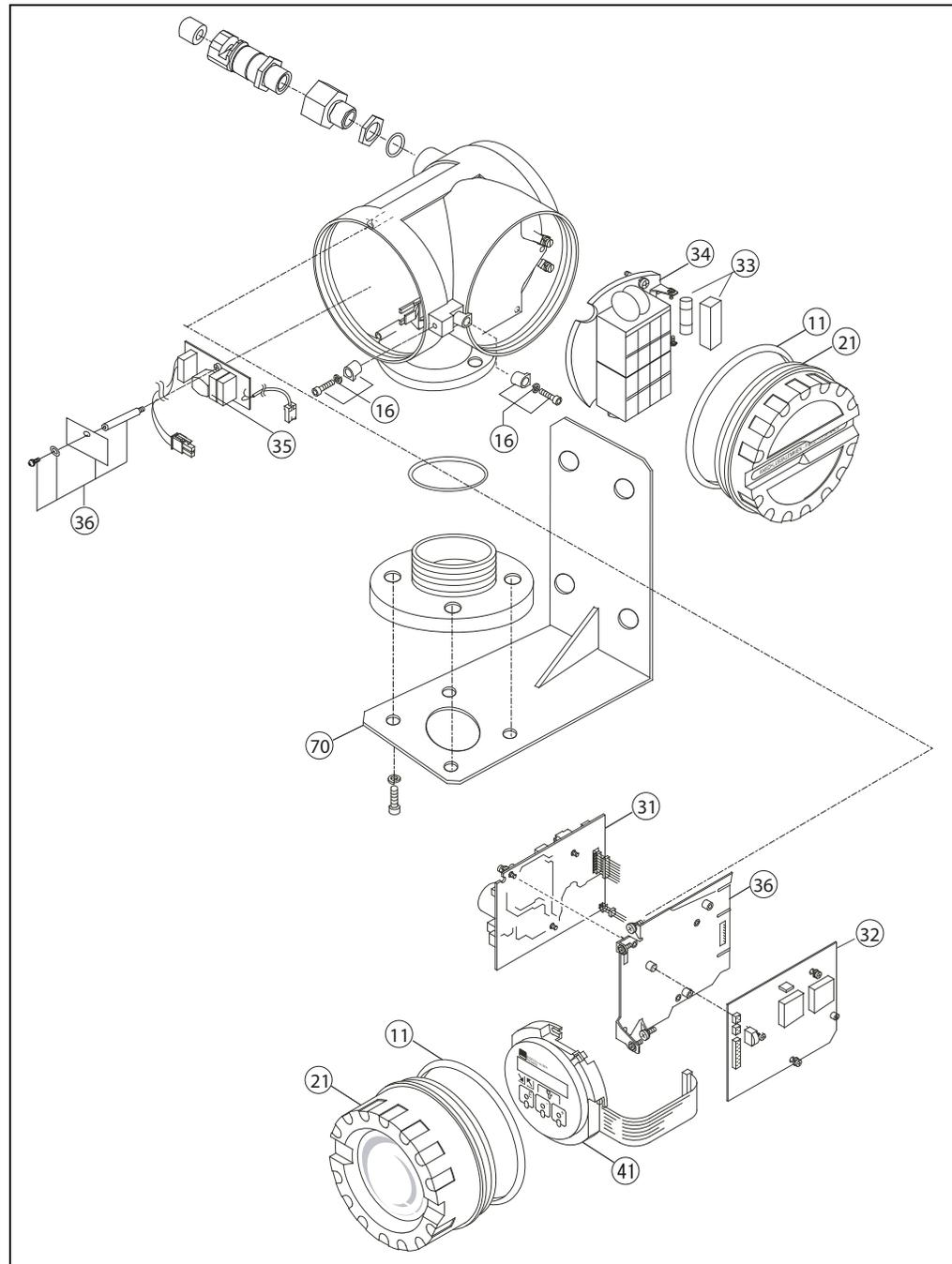
Figure 8-1: 4560 SGM Assembly Diagram
