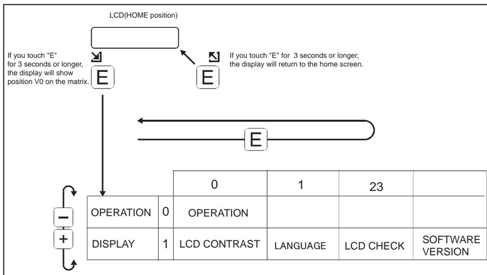
Figure 5-3: Selecting functions within the programming matrix
