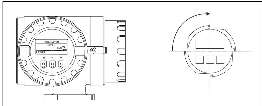
Figure 3-3: Removing or mounting the display and operating elements
