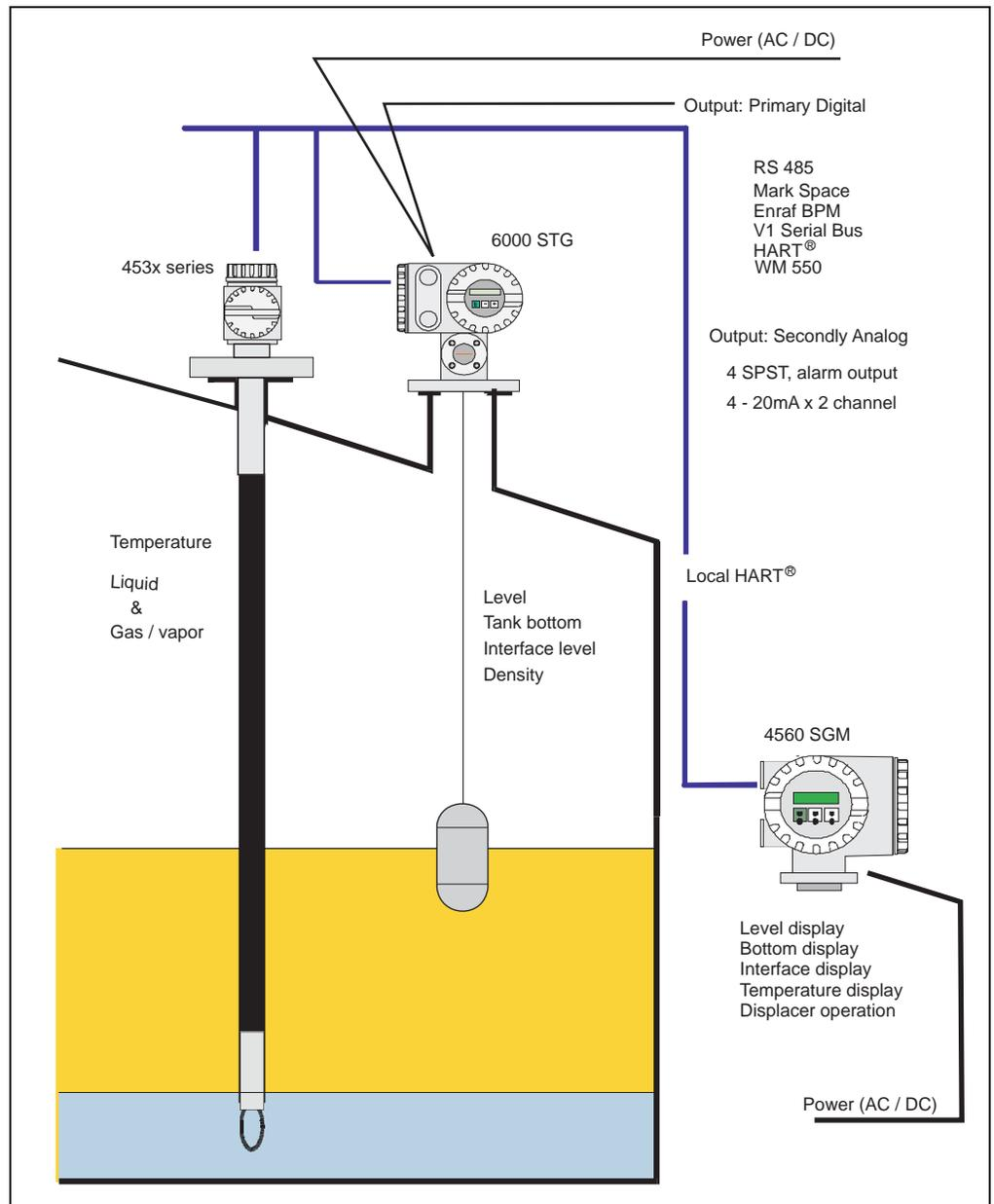
Figure 1-1: Example of a 4560 SGM application
