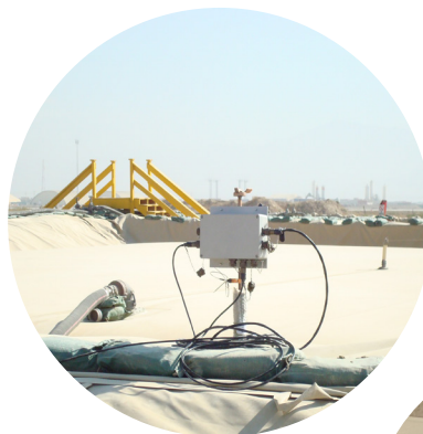
Tactical Data Unit in Theatre used to Collect Pressure and Flow Measurements from Gauges
