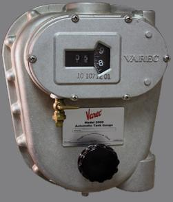
► The N2500 Automatic Tank Gauge (ATG) is a mechanically operated, float and tape instrument designed to provide continuous liquid level measurement in bulk storage applications. Since 1928, over 800,000 units have been sold worldwide, making the N2500 ATG the industry standard for float and tape gauges.
