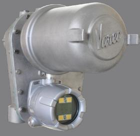
► The N2920 Float & Tape Transmitter (FTT) provides data from the tank side to the control room for use in inventory management applications. It accurately converts mechanical level measurement from the connected tank gauge, integrates temperature and HART devices, and provides digital inputs and digital outputs for the indication of alarms or drive relays.
