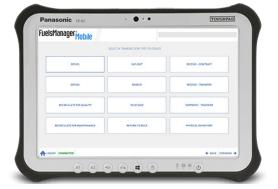
The FuelsManager Mobile Point-of-Sale application runs on a ruggedized tablet and replaces in-the-field data entry as a means of recording fueling transactions. Integrated with other FuelsManager applications, it is an integral part of an automated defense fuels management system that captures inventory and transactions across all fuel points.
