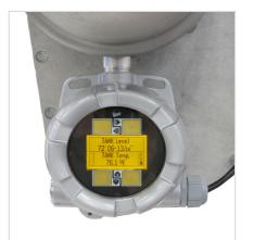
The digital display can be positioned front facing alongside the tank gauge counter display sideways, or rear facing (shown above) underneath the transmitter housing. This allows the transmitter to be installed on existing gauges without having to change their orientation.
