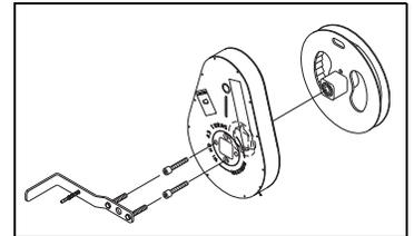
The negator cassette fits all aluminum Varec 2500 (model B & C) Automatic Tank Gauge and can be ordered as an option.
