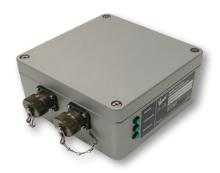
The 8250 Tactical Interface Converter (TIC) provides a communications interface between the Tactical Data Unit (TDU) and the Tactical Mobile Computer (TMC). The 8250 TIC translates data received from the TDU via the RS485 communication protocol, then translates it to an RS232 communication protocol and sends it to the TMC. The TIC also provides continuous DC power to the attached TDUs.
