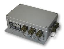
The 8240 Tactical Data Unit (TDU) collects pressure, temperature and meter volume from connected field devices, such as the 7660 Tactical Fuel Gauge (TFG) or a Tactical Flow Meter (TFM). It calculates observed fuel volumes and performs the collapsible tank mapping process. All data is transferred to the TacFuels® Tactical Mobile Computer (TMC) for inventory management and accounting.
