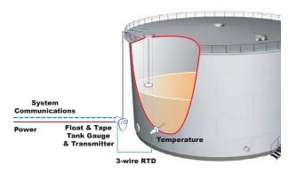
Float and tape gauges work with a variety of tank and product types.
