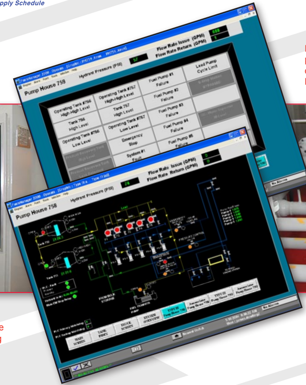
FuelsManager was upgraded and configured to communicate directly with the hydrant fueling system Control Panels
